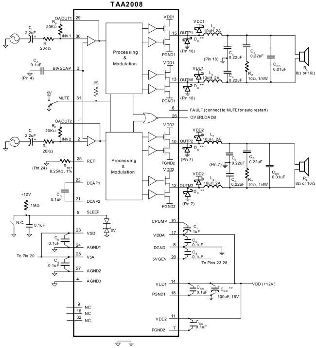
Note: Analog and Digital/Pow er Grounds must be connected locally at the TAA 2008
